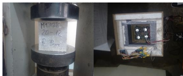
Figure 1. Compressive (left) and thermal conductivity test probe (right).
