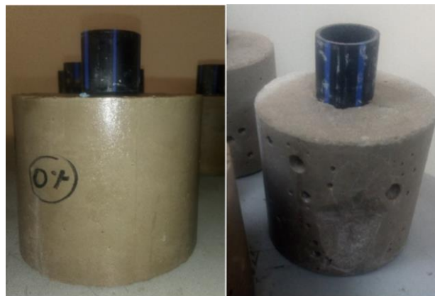
Figure 3. Difference between mortars with and without bentonite. The bentonite content increases the air trapped in the mixture. Left: M_{B,0} , Right: M_{B,5} .
