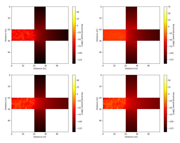
**Figure 5.** Heat map for the isotropic antenna (**top left**), beamforming with mutation strategy-based particle swarm optimization algorithm (MSCPSO) (**top right**), beamforming with the GA (**bottom left**), and beamforming with neuroevolution of augmenting topologies (NEAT) (**bottom right**).
