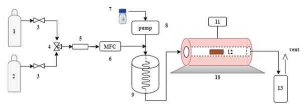
**Figure 2.** Schematic diagram of the experimental setup. (1)  $N_2$ . (2)  $CO_2$ . (3) On-off valve. (4) 3-way valve. (5) Filter. (6) Mass flow controller. (7) Water. (8) Peristaltic pump. (9) Steam generator. (10) Oven. (11) Temperature controller. (12) Sample. (13) Condenser.
