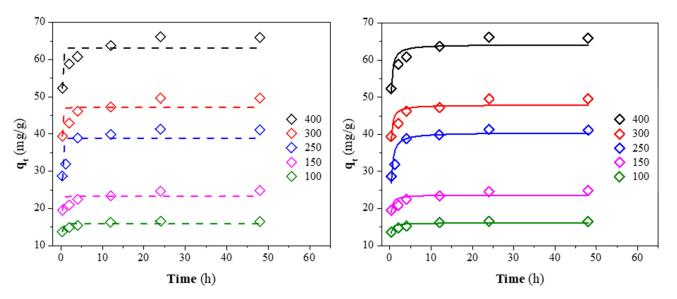
**Figure 10.** Pseudo-first (dash line) and second-order (solid line) kinetic fit for CV on CQW-CO<sub>2</sub> at different initial concentrations.
