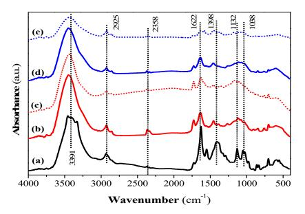
Figure 6. FT-IR spectra of QS-P (a), QS-CO<sub>2</sub> (b), QS-CO<sub>2</sub> CV (c), QS-H<sub>2</sub>O (d), and QS-H<sub>2</sub>O CV (e).
