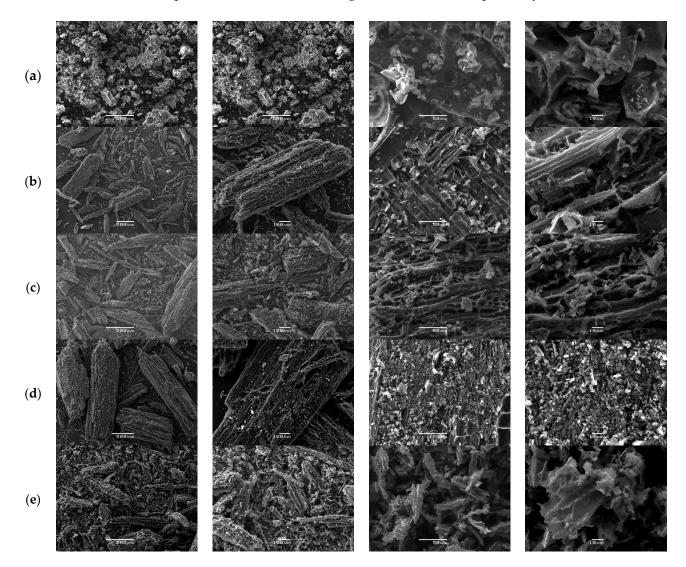
**Figure 8.** SEM images of the QS-P (a), QS-CO<sub>2</sub> (b), QS-CO<sub>2</sub> CV (c), QS-H<sub>2</sub>O (d), and QS-H<sub>2</sub>O CV (e). All images were taken with a magnification of  $500 \times$ ,  $100 \times$ ,  $50 \times$ , and  $10 \times$ , respectively.
