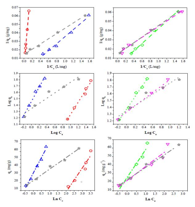
**Figure 9.** Linear fit of experimental data to different isotherm adsorption models. Langmuir (dash line), Freundlich (dot line), Temkin (dash-dot line). QS-H<sub>2</sub>O ( $\diamond$ ), QS-CO<sub>2</sub> ( $\bigtriangledown$ ), CQW-CO<sub>2</sub> ( $\bigstar$ ), CQW-P ( $\triangle$ ), and AC ( $\bigcirc$ ).
