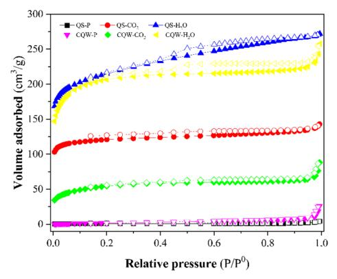
Figure 3. N<sub>2</sub> adsorption-desorption isotherms curves at 196  $^{\circ}$ C of samples. Closed symbols: N<sub>2</sub> adsorption curve and open symbols: N<sub>2</sub> desorption curve.
