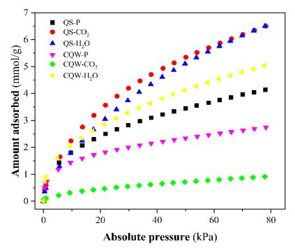
Figure 4. NH<sub>3</sub> adsorption isotherms at 20 °C of the prepared samples.
