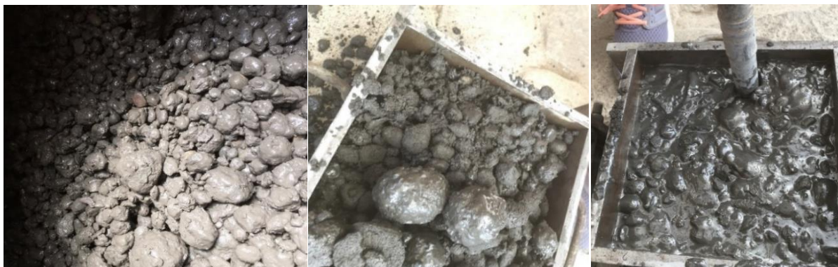
Figure 2. Appearance of the mixture at different stages of preparation. Left: Ash spheres formed during mixing. Center: Ash spheres during mold filling. Right: Appearance of the mixture after vibration.
